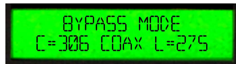
Figure 3.2: Example Bypass Mode Display
